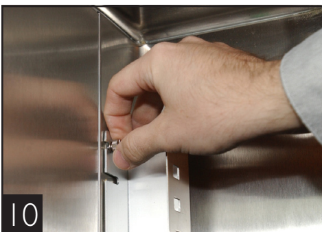
Pilaster installation (side wall of cabinet)
