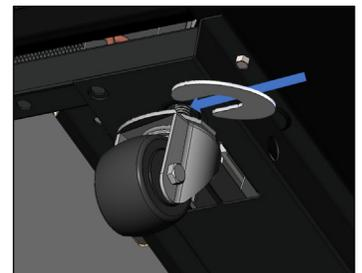
Fig. 7. Install shim(s).
