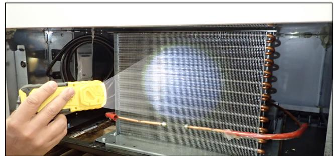
Fig. 3. Verify all blockages have been removed.
