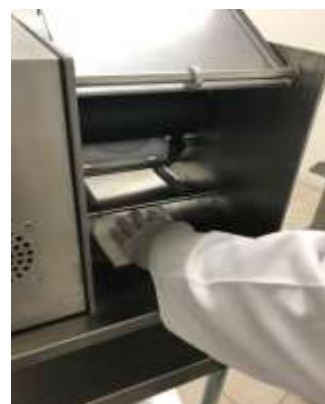
Step 3: Clean around and underneath the rollers.
