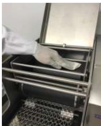
Step 2: Proceed to clean the back roller.
