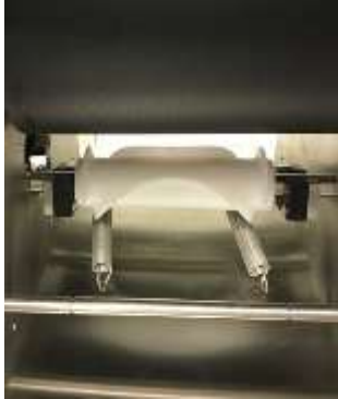
Remove/Release the springs connecting to the silver bar.
