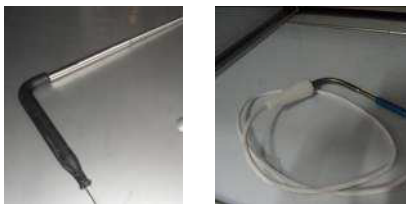
Figure 2: NTC Needle Probe Types
