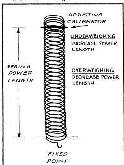
approximately 1/4 turn. This correction must be made equally on BOTH springs. Then, re-set the zero and check the scale at full capacity. Repeat this operation until correct weighing is restored, keeping in mind that, after each spring adjustment, the "zero" balance must be re-set before test weighing.
