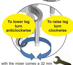
Together with the mixer comes a 32 mm fixed spanner to be used for adjustments.
