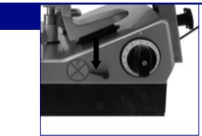
Remove the depositing arm and the chain frame (see section 5.1, page 30)
