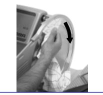
• Turn the blade and disposable cloth with hands for one rotation by slightly pressing the cloth against the guard ring inner side.
