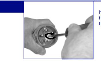
If the direction of rotation is incorrect, reverse the polarity of the phase converter on the three–phase plug of the machine.
