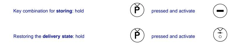
The program stored last before the machine is switched off will become active (startup program) when restarting the machine.
