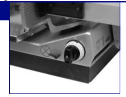
The setting is made by means of the slice thickness **control knob**.
