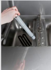
Remove the overflow pipe
