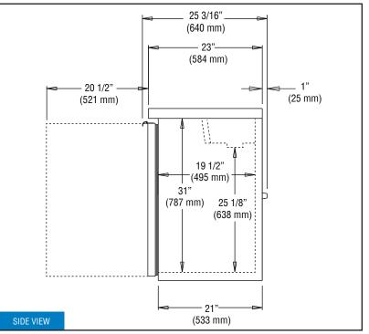
**IMPORTANT NOTE:** Models are completely front breathing and take in and exhaust air through the front grill. For proper operation, the area in front of the cabinet <u>must</u> not be obstructed in any way. A clearance of 1" on the back and 3" on the sides is recommended.
