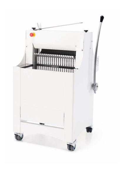
Floor Model Bread Slicer, Up To (250) Loaves Per Hour, Crumb Drawer, Mechanically Assisted Infeed, Automatic Stop, Casters (2 with Locks), 2/3 HP, 120V/60/1P/6A, NEMA 5-15P, cETLus
