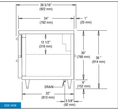
IMPORTANT NOTE: If the cabinet is located directly against a wall, a <u>minimum clearance of 3" is required</u> on sides, front and rear. 1" NPS Drain Tube must be directly piped to a building floor drain or connected to a suitable waste line.
