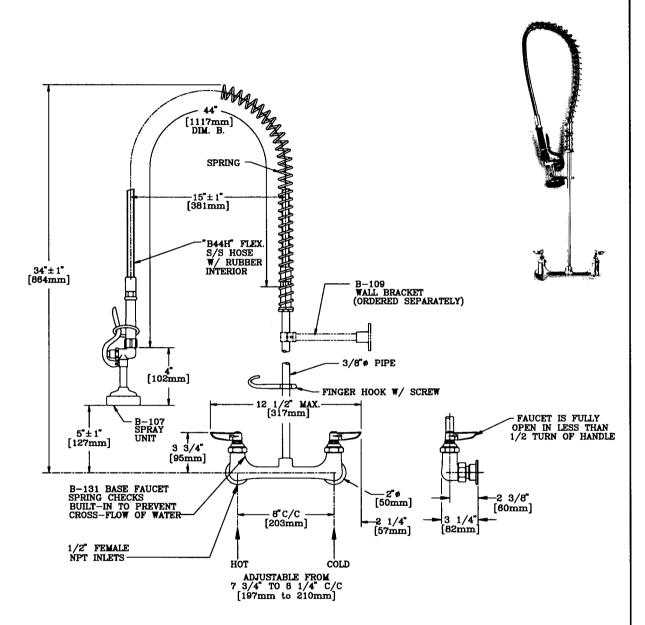
NOTE: ALSO AVAILABLE WITH 1/2" NPT MALE INLETS AND LOCKNUTS ON FAUCETS IN PLACE OF FEMALE INLETS.
