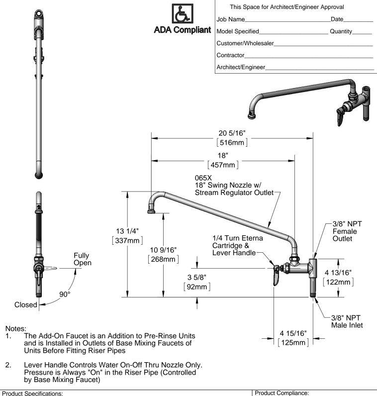
Add-On Faucet w/ 1/4 Turn Eterna Cartridge, Lever Handle & 18" Swing Nozzle w/ Stream Regulator Outlet
