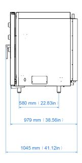
\* Oven must be installed a minimum of 19.7" (500 mm) from any significant source of heat and/or grease (for example: fryers, burners, kettles, open flames, etc.)
