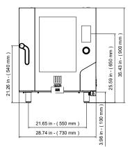
\* Oven must be installed a minimum of 19.7" (500 mm) from any significant source of heat and/or grease (for example: fryers, burners, kettles, open flames, etc.)
