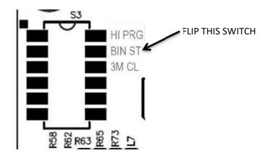
**Note:** Adjust Bin Thermostat so that ice level is maintained in bin at level of thermal well according to directions below.
