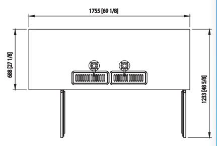
Barrels(1/2) 3 Capacity 23 Cu.Ft. Doors 2 Refrigerant R-290 Temperature 33°F ~ 39°F Range Sliding Easy Maintenance Condensing Unit 9.8 ft long (3m) flexible three Connection wire cord with modeled plug HP 3/8 Voltage 115V/60Hz **Amps** 3.8 NEMA Config. NEMA 5-15 Lighting Interior LED lighting
