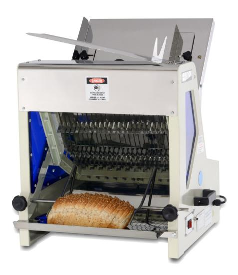
Bread Slicer, Electric, Countertop, Loaves Up To 5" (127mm) High, 5/8" Thick, 15" Wide Blade Holder, 22" Infeed Chute, 1/4 HP, 120V/60/1P/6A/0.7kW, NEMA 5-15P, cETLus (Not Designed for Artisan Style Breads)
