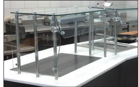
10-1/2" Standard Glass Opening (Maximum 13") From Table To Bottom Of Glass. Max. Load For Top ism 100 Lbs. Evenly Distributed Wt.
