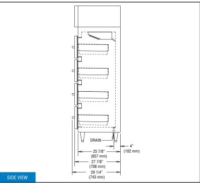
IMPORTANT NOTE: If the cabinet is located directly against a wall and/or under a low ceiling, a minimum clearance of 12" is required on top and 3" on sides and rear. 1" NPS Drain Tube must be directly piped to a building floor drain or connected to a suitable waste line.
