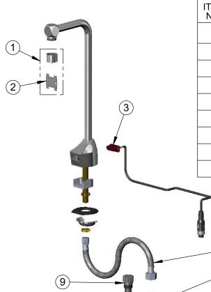
ITEM DESCRIPTION SALES NO. NO. VR 1.5 GPM Laminar Flow Device (Anti-Microbial) 1 B-0199-06-LF15A w/ VR Key 2 015425-45 Vandal Resistant Key 3 019174-45 Sensor Cable Asssembly 4 016297-45 Inlet Hose, Faucet, 1/2" NPSM-F x 1/4" NPSM-F 5 ChekPoint Control Module w/ Filter Tee 019944-45 6 5EF-0002C AC Adapter - US Plug 7 5EF-0005 Supply Hose, 9/16-24 Female x 1/2" NPSM 8 002534-25 Close Nipple, 1/2" NPT 9 **EC-FILTER** Replacement Filter
