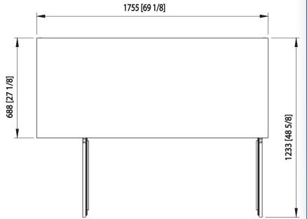
2 Door Capacity 23.4 Cu.Ft. Shelves Refrigerant R-290 Temperature 33°F ~ 39°F Range Sliding Easy Maintenance Condensing Unit 9.8 ft long (3m) flexible three Connection wire cord with modeled plug HP 3/8 Voltage 115V/60Hz **Amps** 3.8 **NEMA** Config. NEMA 5-15 Lighting Interior LED lighting
