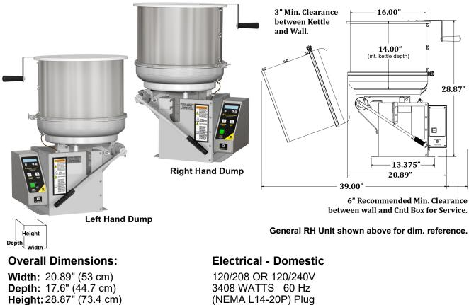
Reference drawing shown for additional dimensions and clearances required.
