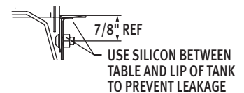
Sectional View Showing Table Connections
