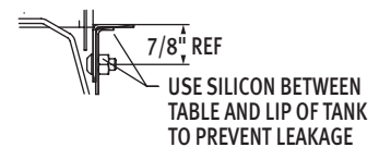
Sectional View Showing Table Connections
