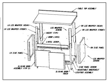
(1) Attach leg/foot assemblies to the adjustable undershelf. Leave 6" from the bottom of casting to bottom of leg (as shown).
