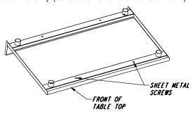
(6) Re-install the sheet metal screws thru the designated holes in the lintel. The holes should match with leg channel holes (diagram shows back side of lintel).
