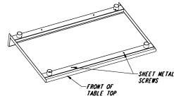
(6) Secure table top to legs by tightening set screw with allen (hex) wrench. Typical (4) places (lintel not shown for clarity).
