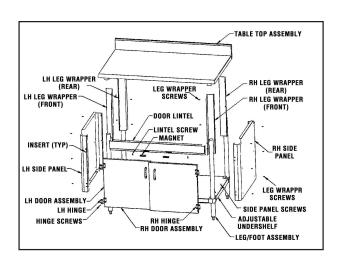
(2) Slide side panels over leg/foot assemblies and attach with screws.
