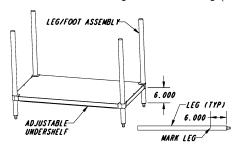
(2) Slide side panels over leg/foot assemblies and attach with screws.
