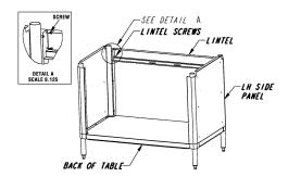
(5) Secure table top to legs by tightening set screw with allen (hex) wrench. Typical (4) places (lintel not shown for clarity).
