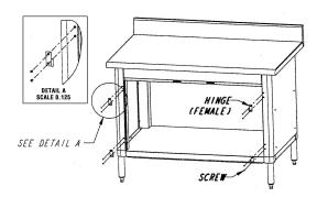
(12) Install right and left hand door assemblies by sliding (male) pinned hinges on doors to female hinges on side panels.
