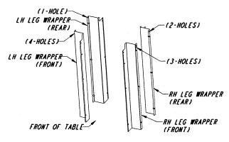
(8) Diagram shows all leg wrappers in place with screw placements. Six screws secure each leg wrapper (some screws not shown).
