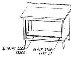
(10) Install sliding doors by placing them behind the lintel into their separate tracks. Lift up on the bottom of the door to clear bottom track and place in corresponding track. (Place door in rear track first.)
