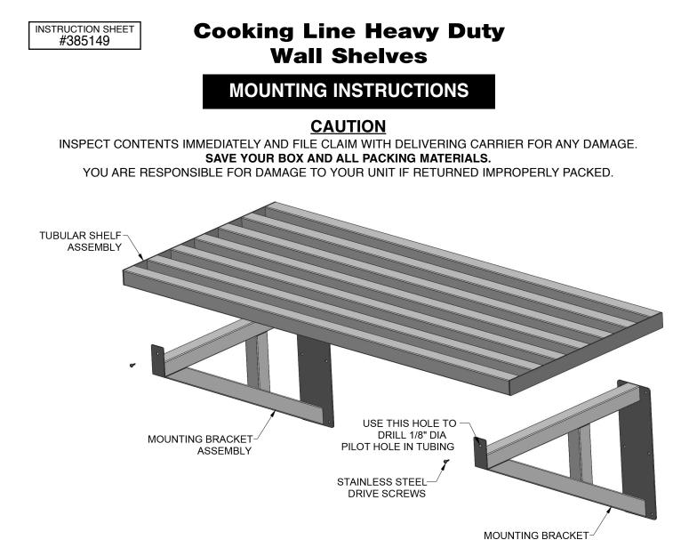
Prior to mounting your shelf, verify that you have sufficient structural support in the wall to be able to properly hold the shelf and its contents.
