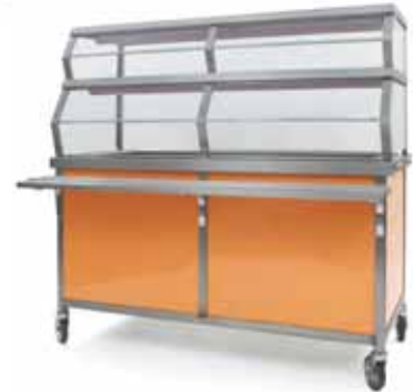
Cold food unit shown with optional double tiered glass sneeze guard with florescent lamps, optional tray slide, optional orange laminate panels, and server side shown with optional louvered doors
