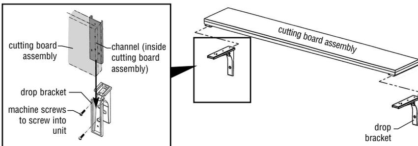
1. Mount drop brackets to table, using machine screws and threaded fasteners on table.
