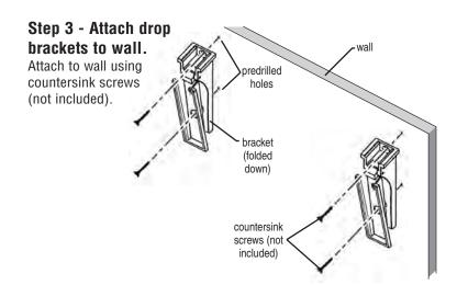
\* IMPORTANT: Wall mounted units must be attached to a properly constructed and sound wall. For walls constructed of wood or steel studs, the mounting points must be directly on the stud or suitable in-wall-grounds of plywood or sheet metal. Eagle Group cannot be held responsible for the failure of the device or any other devices due to improper installation.
