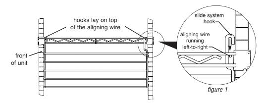
Center slide system under desired shelf. Hook to top of the shelf on the wires that run left-to-right as shown in *figure 1*.
