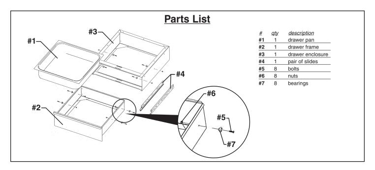
Step 1 - Attach bearings to drawer frame.
