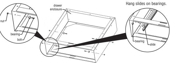
Step 5 - Attach drawer enclosure to hat channels underneath adjoining table.
