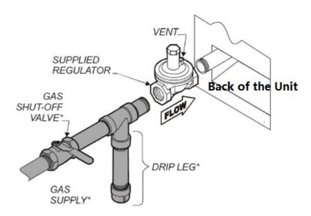
Prior to connecting the regulator, check the incoming line pressure. The regulator can only withstand maximum pressure of ½ PSI (14" WC). If the line pressure is beyond this limit, a step down regulator before the regulator provided will be required. The arrow above(FLOW) shows gas flow direction and should point downstream to the equipment.
