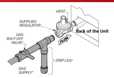
Prior to connecting the regulator, check the incoming line pressure. The regulator can only withstand a maximum pressure of  $\frac{1}{2}$  PSI (14" WC). If the line pressure is beyond this limit, a step down regulator before the regulator provided will be required. The arrow above(FLOW) shows gas flow direction and should point downstream to the equipment.
