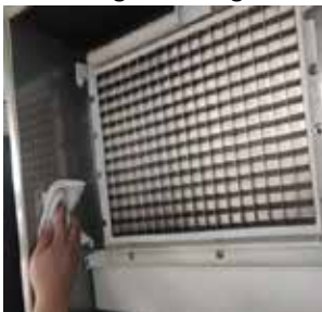
Scrub the inner wall of the ice board
