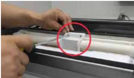
Remove the fixed bracket of the flow pipe
