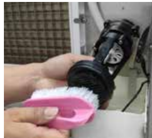
Brush the bottom of the pump
