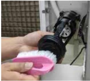
Brush the bottom of the water pump
