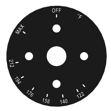
The thermostat is connected to a graduated knob located inside the cooker door. Rotating the knob clockwise to the desired cooking temperature (set¬point) directly adjusts the thermostat to that temperature. The thermostat controls the water tank temperature by regulating the gas supply to the burner via the gas valve.
