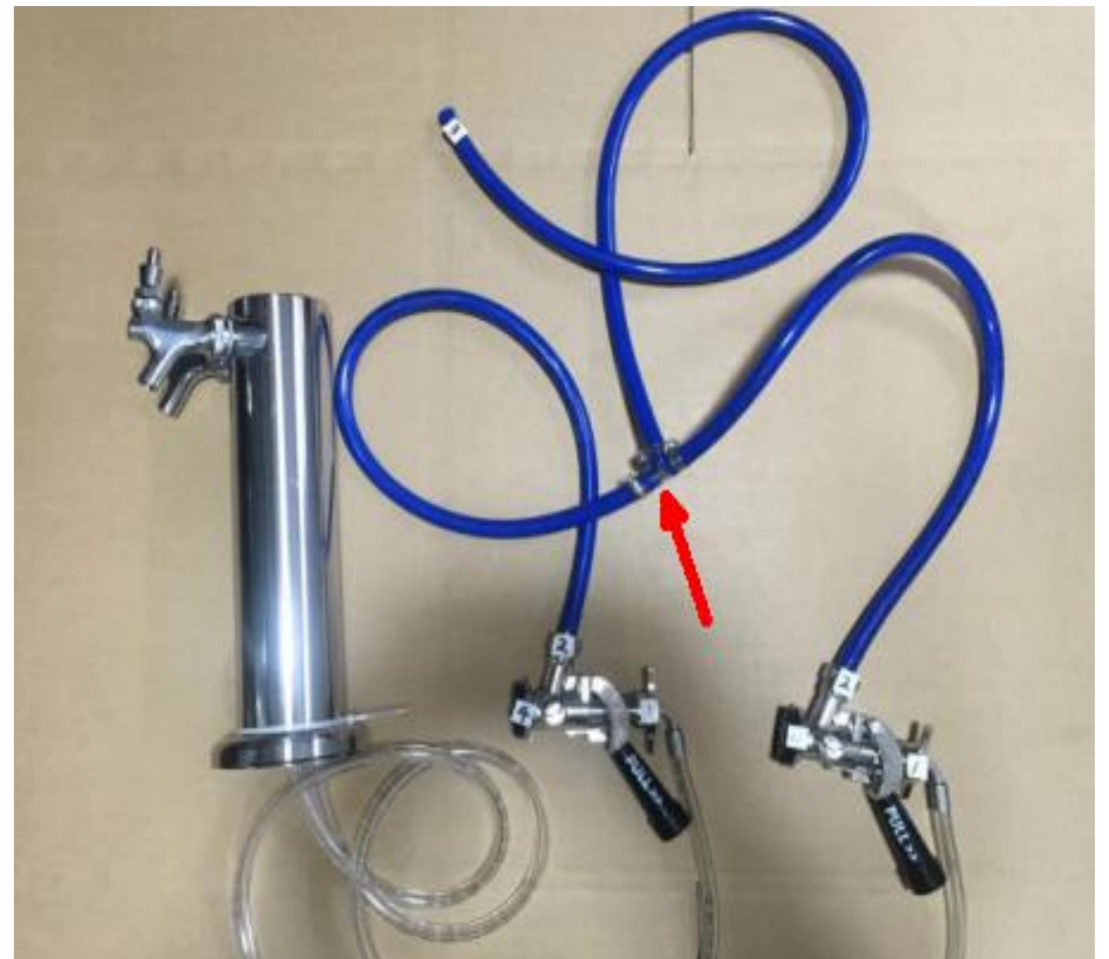
TEE JOINT IS USED TO CONNECT THREE CO 2 TUBE LIKE BELOW:
