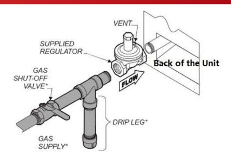
Prior to connecting the regulator, check the incoming line pressure. The regulator can only withstand a maximum pressure of ½ PSI (14" WC). If the line pressure is beyond this limit, a step down regulator before the regulator provided will be required. The arrow above (FLOW) shows gas flow direction and should point downstream to the equipment.
