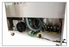
**Pump**3 HP oil rotary pump.
