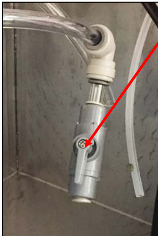
Fig. 2 Priming valve in OPEN position
