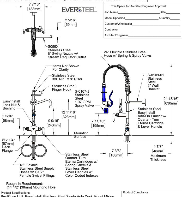
Pre-Rinse Unit: EasyInstall Stainless Steel Single Hole Deck Mount Mixing Faucet, SS Quarter-Turn Eterna Cartridges w/ Spring Checks, SS Lever Handles, SS Add-On Faucet, SS 6" Swing Nozzle, 24" Flexible Stainless Steel Hose, SS 1.07 GPM Spray Valve, SS 6" Wall Bracket & Flexible Stainless Steel Supply Hoses
