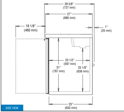
IMPORTANT NOTE: Models are completely front breathing and take in and exhaust air through the front grill. For proper operation, the area in front of the cabinet must not be obstructed in any way. A clearance of 1" on the back and 3" on the sides is recommended.
