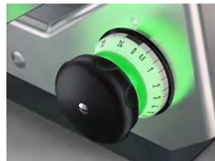
Gauge plate closed, safe for cleaning - green.
