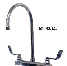
FAUCET AERATOR CONFORM TO ASTM.A112.18.1M • 2.2 GPM/8.3 LPM THREAD: 55/64 - 27 FEMALE
