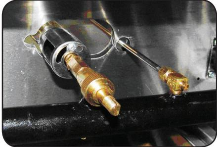
2. Unscrew bolts and pilot valve, then remove the manifold.
