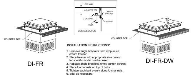
\*Provided hardware allows for unit to be removable as necessary
