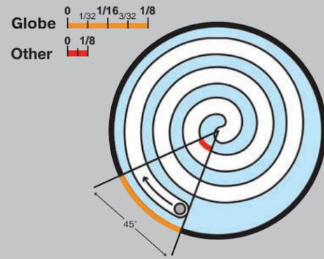
Traditional slicers begin the travel of the seated pin at the center of the cam, moving outward. The S-Series not only bevels the pin and cam path, preventing play caused by gradual wear, but also the travel begins on the outside of the spiral. This simple innovation delivers precise control where it matters most.
