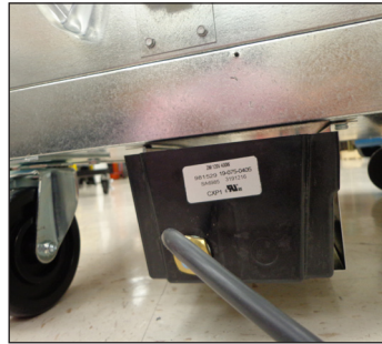
Fig. 4. Place the HDP in the HDP bracket.
