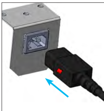
Fig. 1. Fully insert the power cord into the receptacle.
