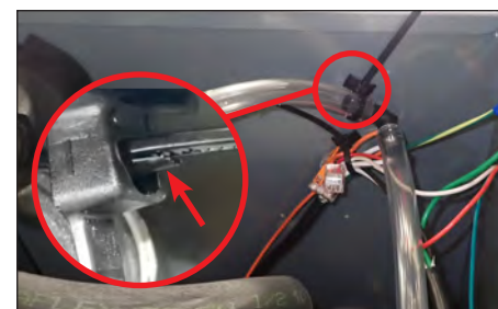
Fig. 3. Cable tie release tab location.
