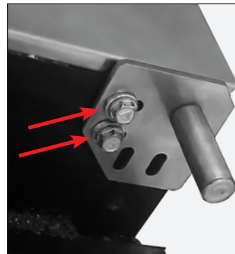
Fig. 9. Do not forget the washers.
