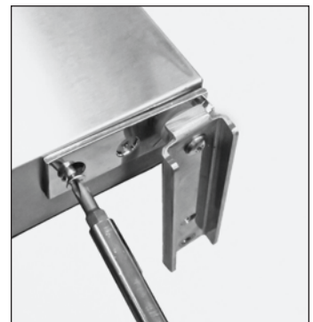
Fig. 5. Remove the cartridge hinge assembly.
