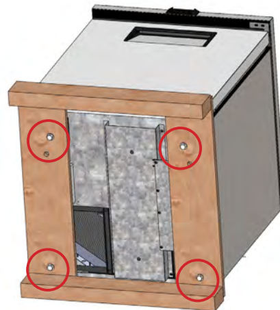
Fig. 3. Remove all shipping bolts.
