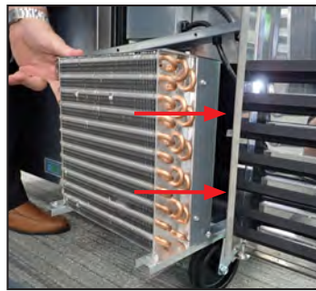
Fig. 7. Carefully slide the condensing unit back into position and replace bolts and coil brackets.
