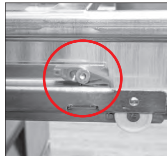
Fig. 5. Drawer retainer location. Retainer is engaged.
